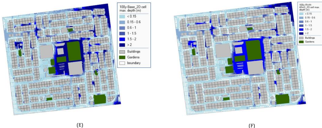
Figure 11: Flood depths for (25, 50 and 100) return periods: (A) 25y flood depths without RWH tanks, (B) 25y flood depths with 24 m 3 RWH, (C) 50y flood depths without RWH tanks, (D) 50y flood depths with 32 m 3 RWH, (E) 100y flood depths without RWH tanks, (F) 100y flood depths with 40 m 3 RWH.
